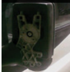
MISSING MIRROR COVER
